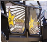
Front door opens suicide, rear door opens standard for more access clearance.
